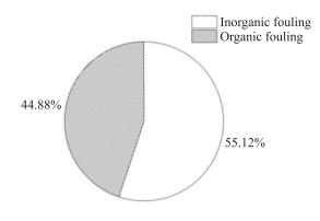
Fig.3. LOI measurement of membrane foulants.
