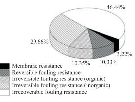
Fig.4. Fouled UF membrane resistance analysis.
