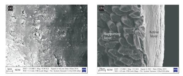
Fig.2. SEM images of the fouled UF membrane: (a) surface (magnification, 8,000×); (b) cross-section (magnification, 512×).
