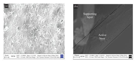
**Fig.5.** SEM images of the fouled UF membrane after chemical cleaning: (a) surface (magnification,  $3,130\times$ ); (b) cross-section (magnification,  $1,060\times$ ).
