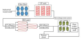
**Fig.1.** Flow diagram of the industrial wastewater purification plant at CSC.
