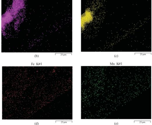
Fig.6. (a) SEM cross-section image and (b-e) the EDS mapping images of the fouled UF membrane after chemical cleaning.
